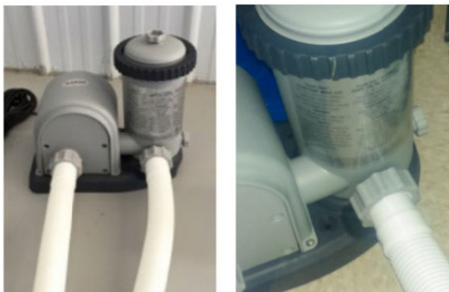
Filter Pump Connection Filter Pump Outlet
