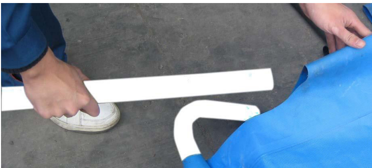
Step 13: Insert the other short framework elbow tube into the liner and attach it to the long connector tube.
