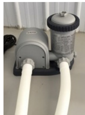
Filter Pump Connection
