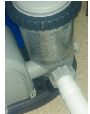
Filter Pump Outlet
